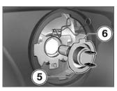
• Insert bulb **5** while ensuring correct position of lug **6**.
